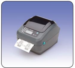
The direct thermal GX420d is extra compact to fit in congested workspaces and produces 203-dpi print resolution at speeds up to 6 inches per second. Its wide range of options include 802.11b/g or Bluetooth® wireless connectivity and 10/100 Ethernet, in addition to standard USB/serial/parallel. Increase your media choices and application flexibility with cutter, peeler, and adjustable black line sensor options.
